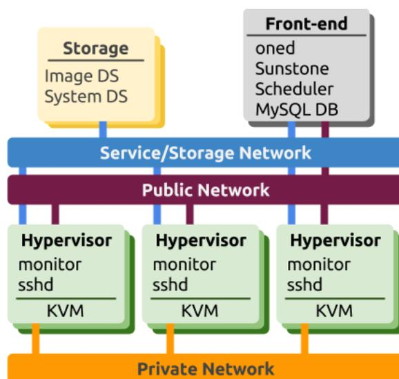
**Figure 1.** Reference Architecture, a bird's eye view
