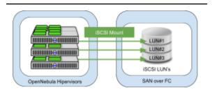
Hypervisor hosts will locally mount an independent LUN device exported by SAN using the iSCSI protocol. OpenNebula local storage drivers with qcow2 image format support provide full storage functionalities, including cold/live migration, system snapshots, and thin provisioning.
