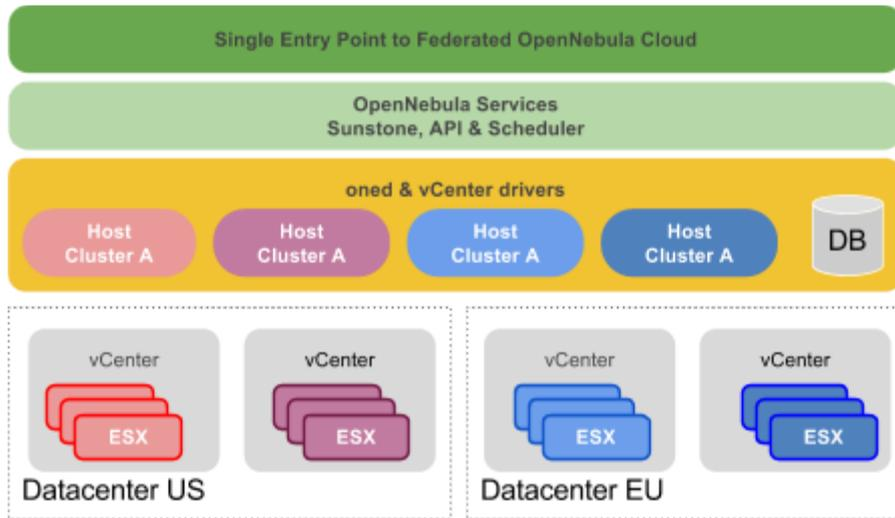
**Figure 4.** Single OpenNebula multi-datacenter deployment
