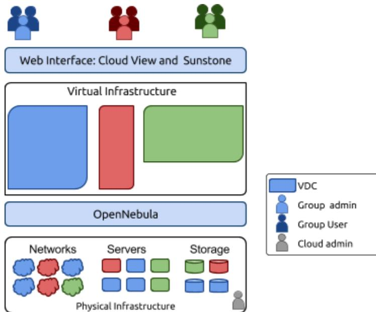
**Figure 3:** Resource Provisioning Model in OpenNebula
