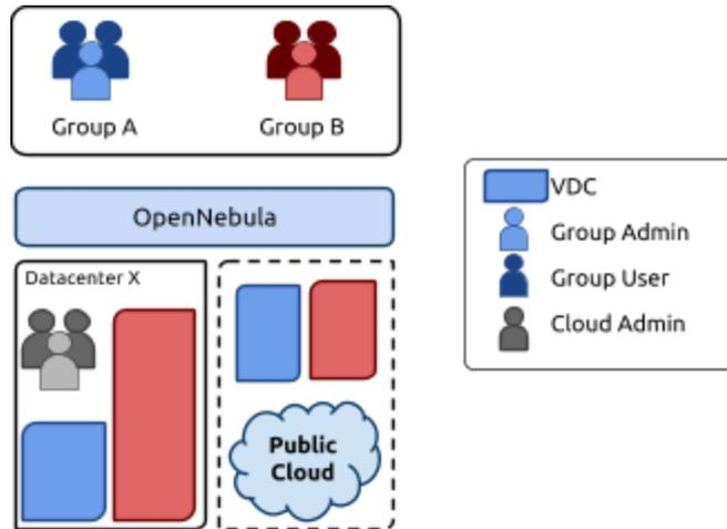
**Figure 6:** Hybrid Cloud architecture enabling cloud bursting
