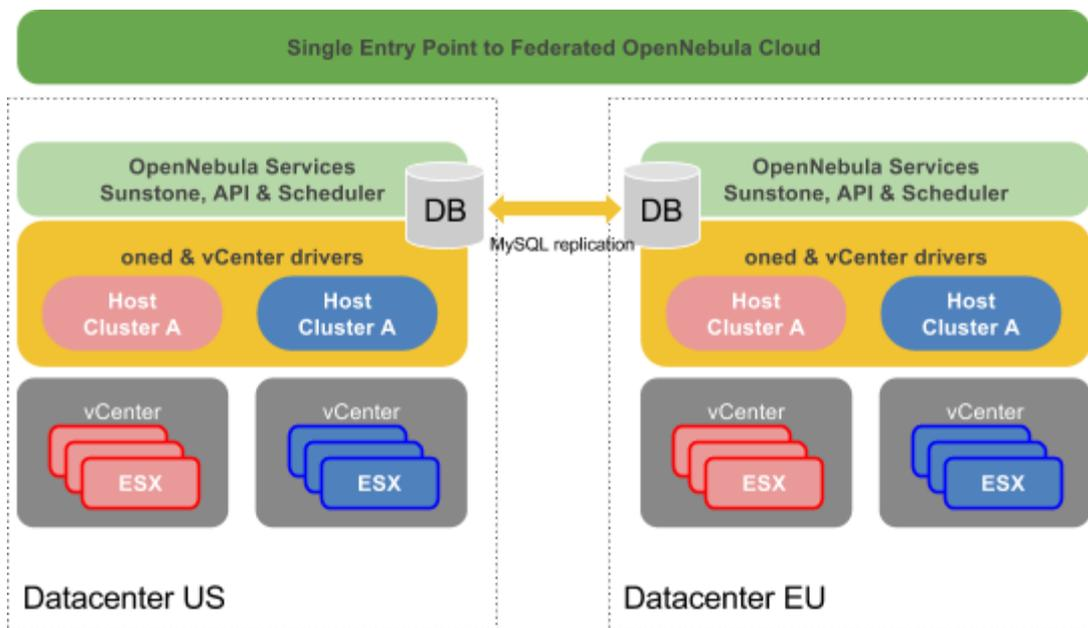
**Figure 5.** Multi-datacenter deployment based on two OpenNebula zones
