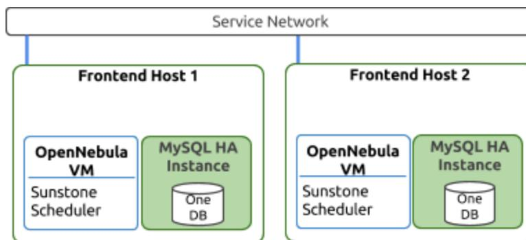
**Figure 7:** Overview of the HA architecture and main components
