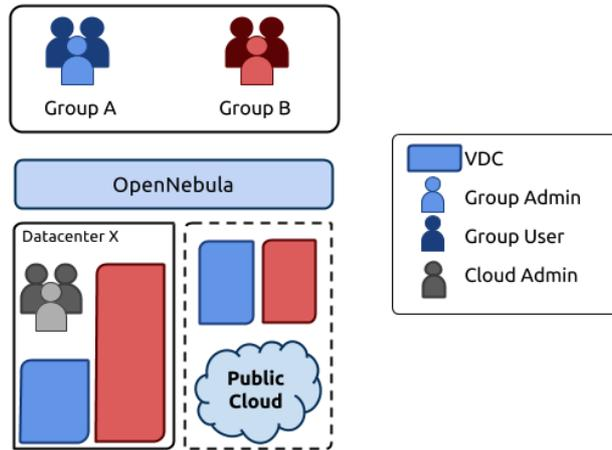
Figure 5: Hybrid Cloud architecture enabling cloud bursting
